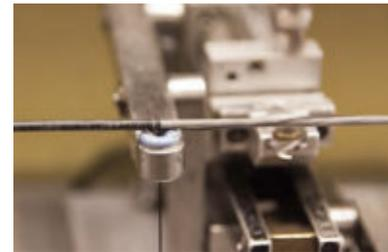
The LiveWire™ machine then wraps the string under full load, serving throughout the entire process at tensions previously impossible to achieve.
