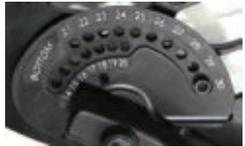
To adjust draw length, simply place the screw in the draw length desired on each cam
